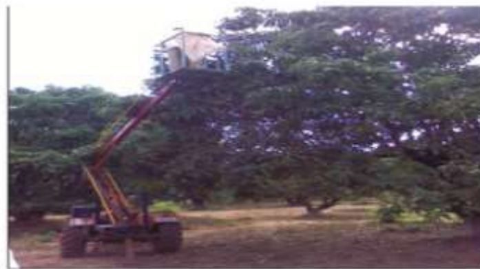
Fig. 1b)Tractor Mounted Hydraulic elevator for harvesting of Mango orchards.
